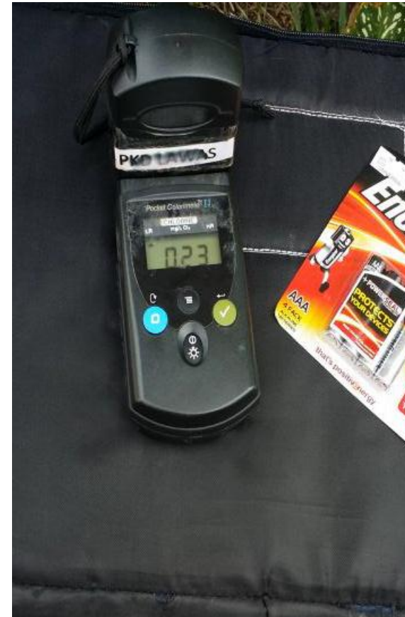
Free chlorine at terminal water more than 50km away from WTP: 0.23 ppm
